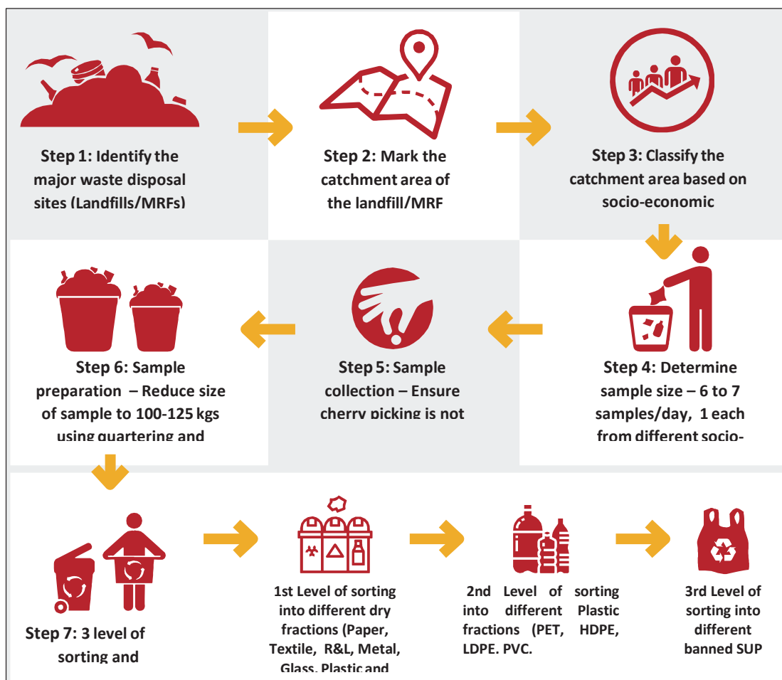
Figure 3: Methodology for quantification and characterisation of SUP in municipal waste
